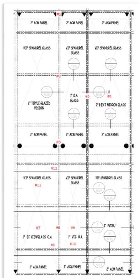
Figure 14. Elevation Showing Transducer Locations for Mock-up
