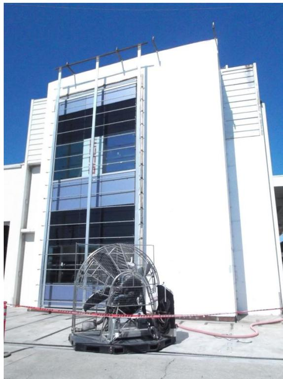
Figure 13. Curtainwall Performance Mock-up Configuration
