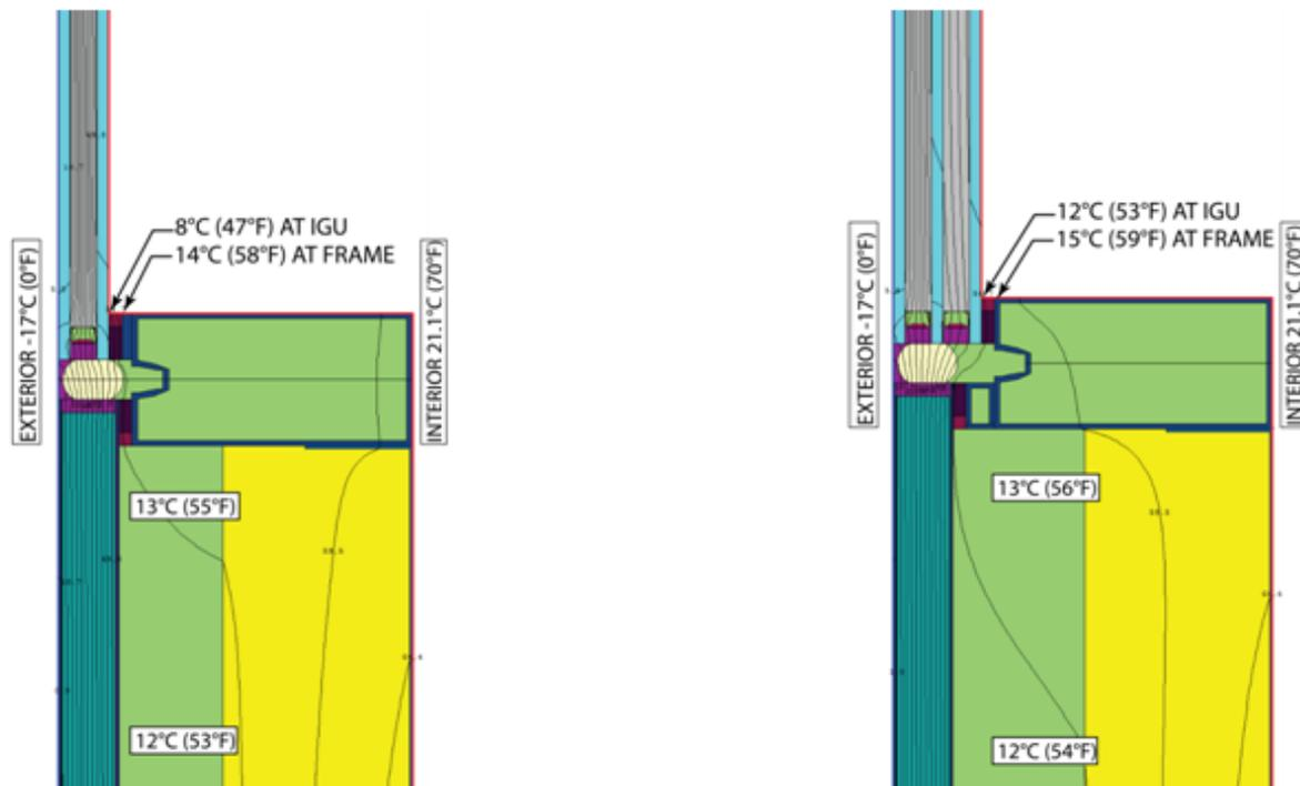
Figure 6. Double and Triple glazing using a combination of VIP's and mineral wool
