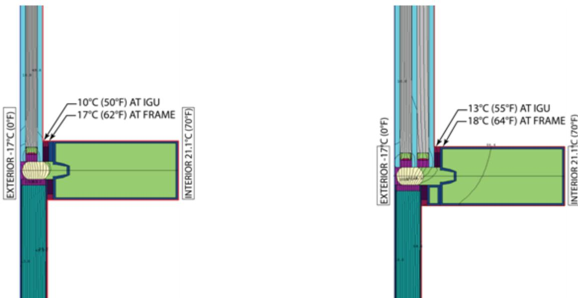
Figure 5. Double and Triple glazing using metal clad VIP's as the spandrel panels
