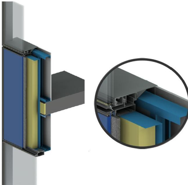
Figure 11 Unitized curtainwall using Triple Glaze AIM
