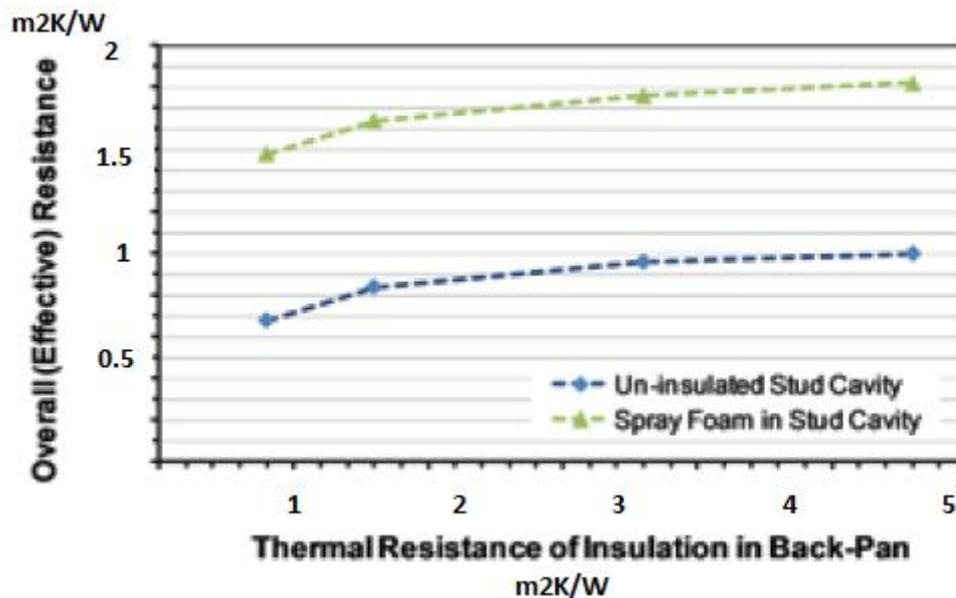
Figure 2 [2]. Diminishing Rate of Return of Spandrel Section with increased insulation
