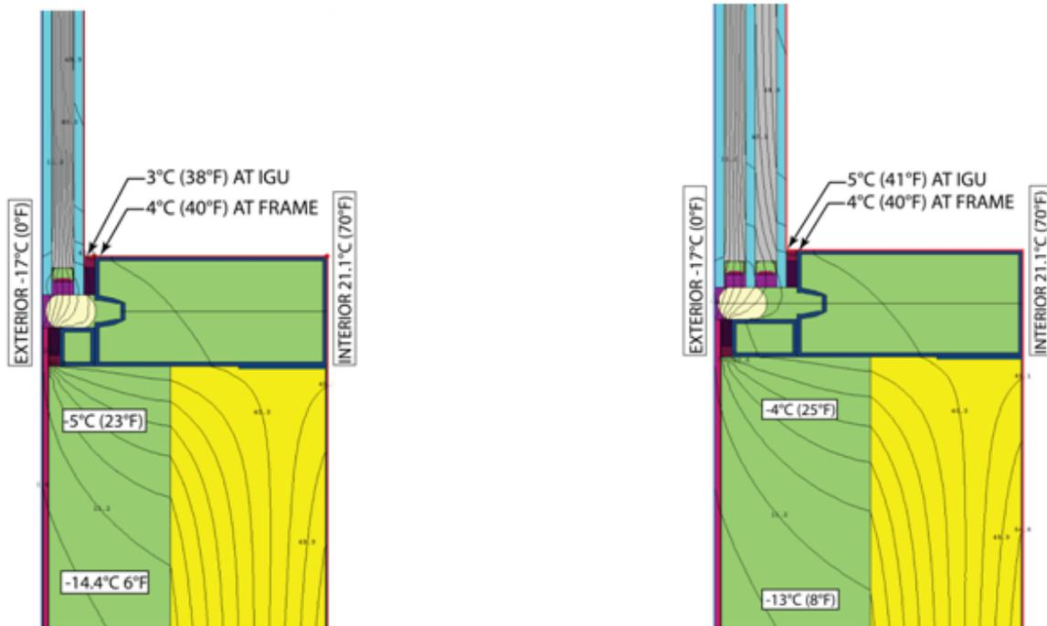
Figure 4. Double and Triple glazing in conventional curtainwall application using mineral wool
