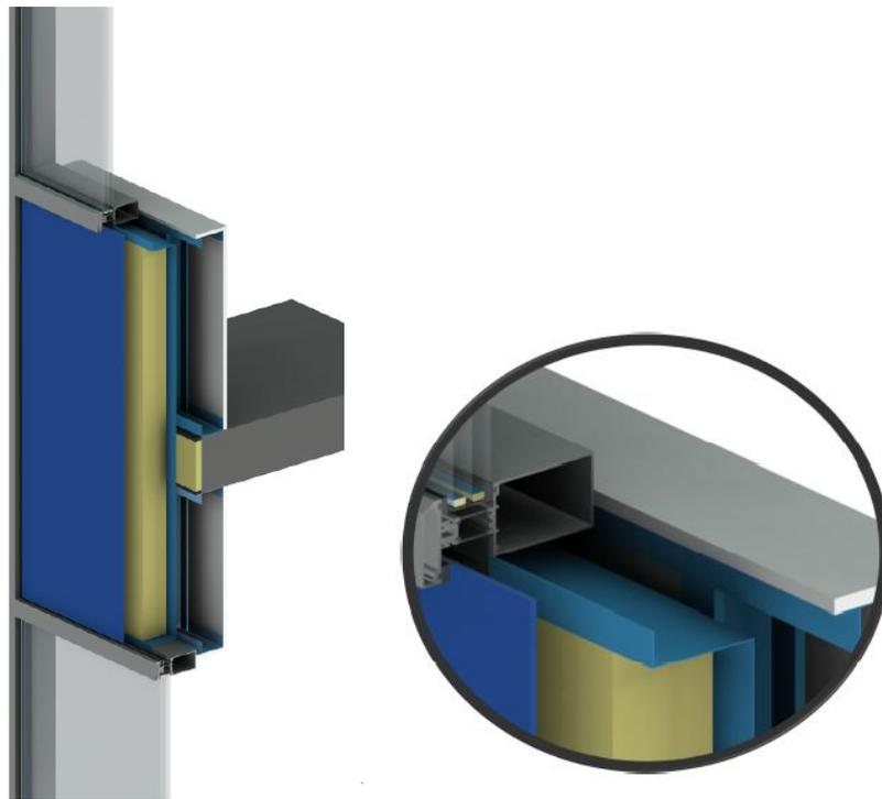
Figure 3. Spandrel section of High Performance Curtainwall
