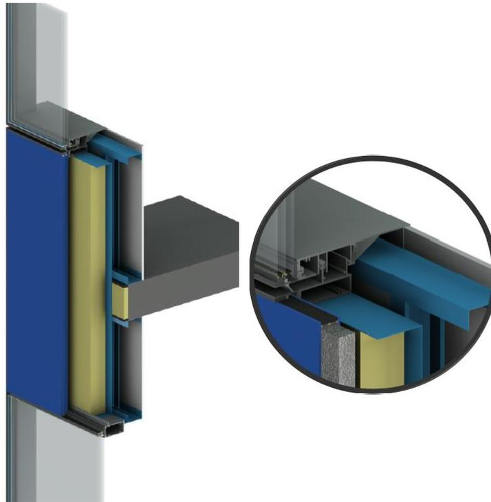
Figure 9. Benchmark Unitized Curtainwall using Triple glazing in both vision and spandrel
