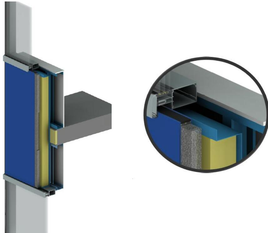
Figure 8. Conventional curtainwall with addition of the double glaze AIM.
