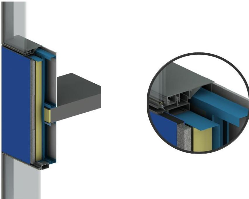
Figure 10. Unitized curtainwall using Double Glaze AIM
