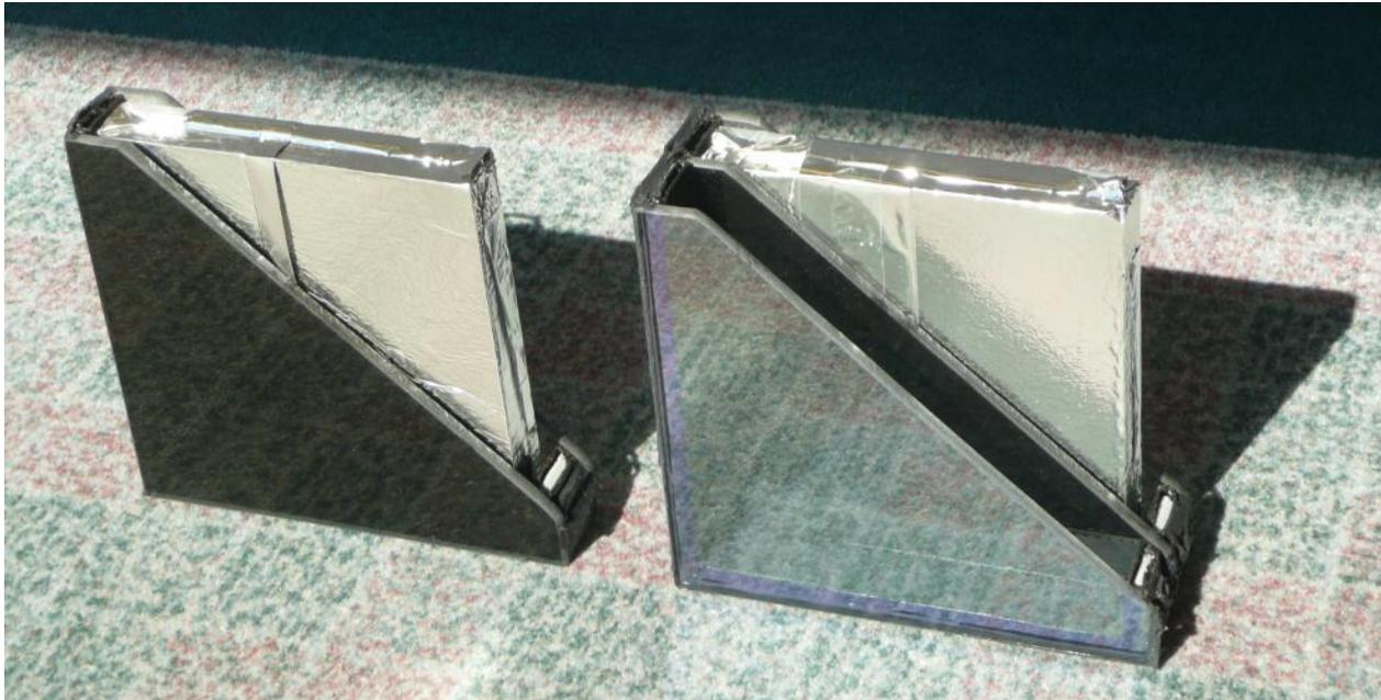
Figure 7. Double Glaze AIM with ceramic frit on surface 2 and Triple Glaze AIM with Low E on surface 2 and ceramic frit on surface 4.
