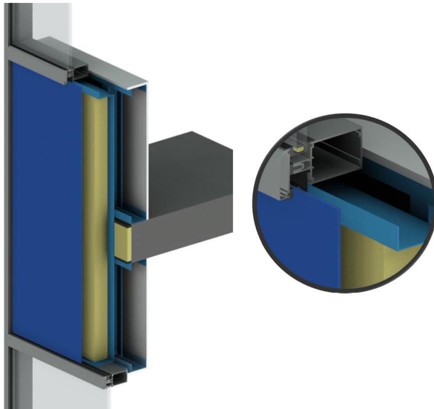
Figure 1. Typical Conventional Stick Curtainwall
